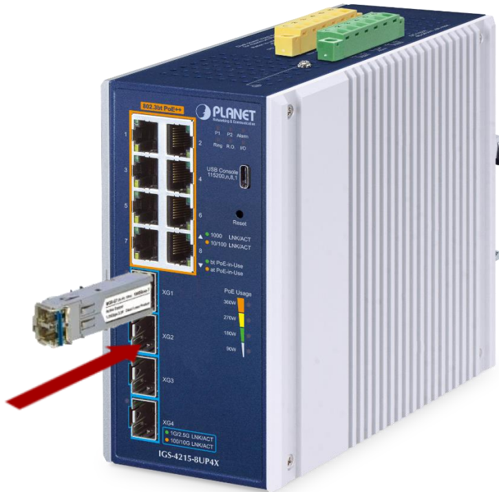
Figure 2-2-4: Plug in the SFP Transceiver
